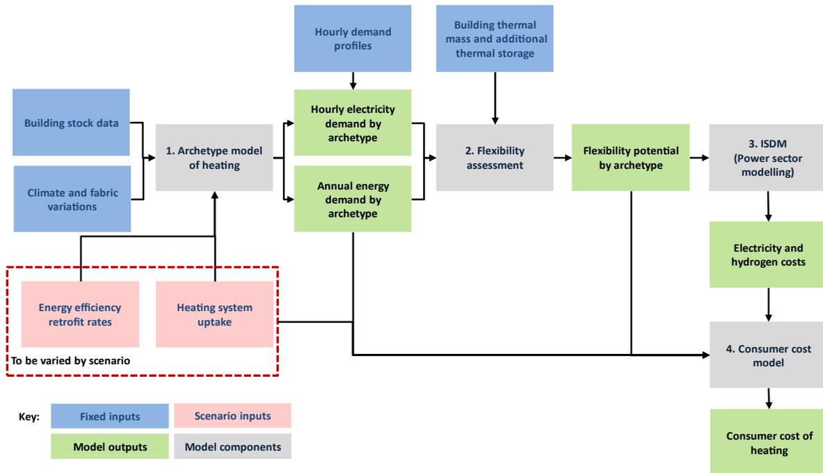
Figure 2 - Full heating system costing model flowchart.
