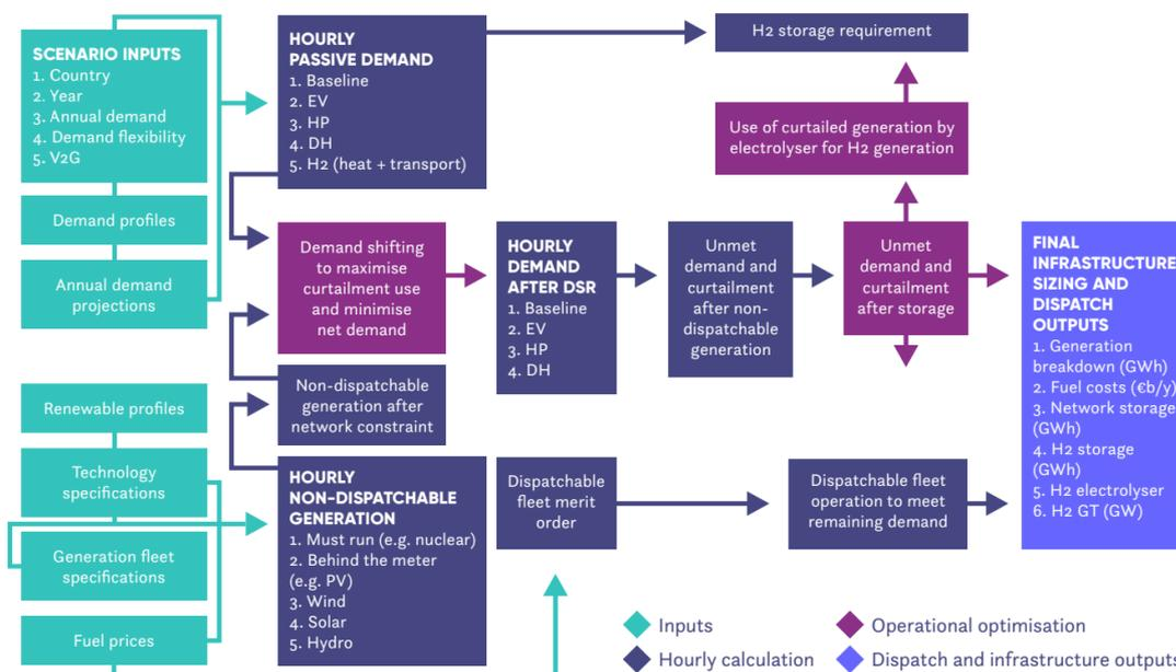
Figure 3 – Schematic of the calculation within the ISDM
