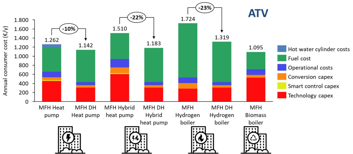
Figure 28 - District heating and building level technology cost for consumers, district heating plant and network costs are included in the fuel cost in valley climate.
