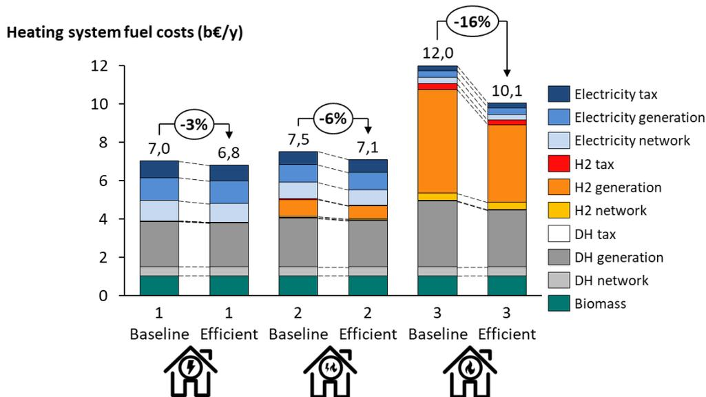
Figure 25 - Fuel cost savings from operating the electricity system in a flexible way (costs shown from system perspective).
