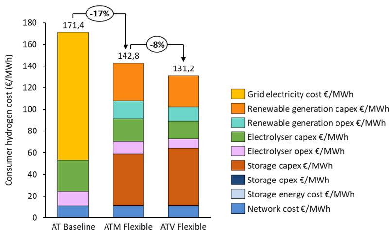
Figure 5 - Cost of hydrogen for consumers in the baseline case, which applies to both ATM and ATV, and in the flexible case for each climate region separately
