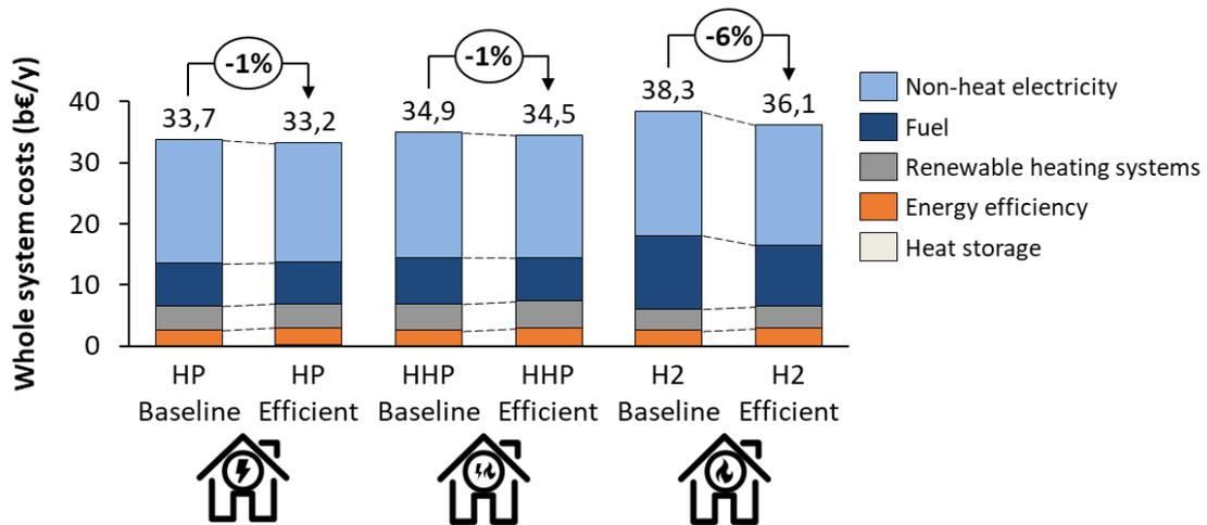
Figure 14 - The system cost saving from the efficient scenario in Austria.
