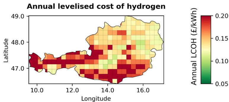
Figure 4 – Levelised cost of hydrogen production modelled across Austria using electrolysers co-located with on-shore wind
